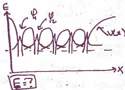
Use a basis of  $\psi$  function at each atom and ~~diagonalize~~ diagonalize
