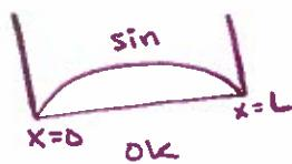
$$\Rightarrow \psi_n(L) = 0 = \sin \sqrt{\frac{2meE_n}{\hbar^2}} L \Rightarrow \sqrt{\frac{2meE_n}{\hbar^2}} L = n\pi \quad n=1, 2, 3, \dots$$
