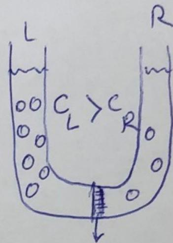
membrane impermeable to particles (except solvent)
